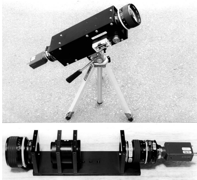
Figure 1 – The TV observation equipment. The device with the Image Intensifier (Delft High Tech XX1470 etc.).
